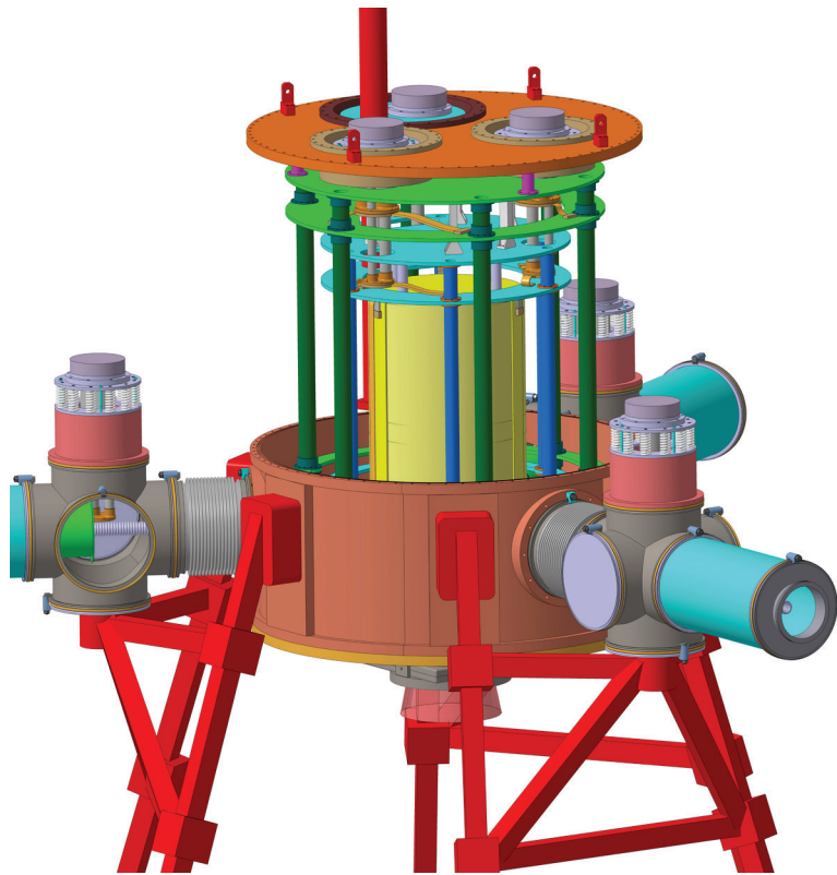
Conceptual scheme of the cryostat for testing and calibrating the Focal Plane Assembly of Athena /X-IFU. Credit: INTA – C2CC team.
