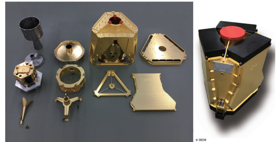
Left: The various sub-assemblies of the FPA-DM during integration. At the top left the Niobium shield is shown. The triangle in centre is one of three Kevlar cord assemblies which together form the suspension of the T_1 stage. The hexagonal structure on the left is the partially assembled detector stage. Right: The FPA-DM #1 completely assembled. The front-side red cap is a protective cover to avoid contamination of the optical filter. The three front black covers will be replaced by the readout harness during further tests. The black back-side cover protects the sensitive electronics and internal harness of the FPA during transport and handling.
