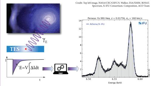
The energy deposited by an X-ray photon is converted into a current pulse (left). Software algorithms on-board analyse the pulse and estimate the energy of the incoming photon to create a spectrum (right).
